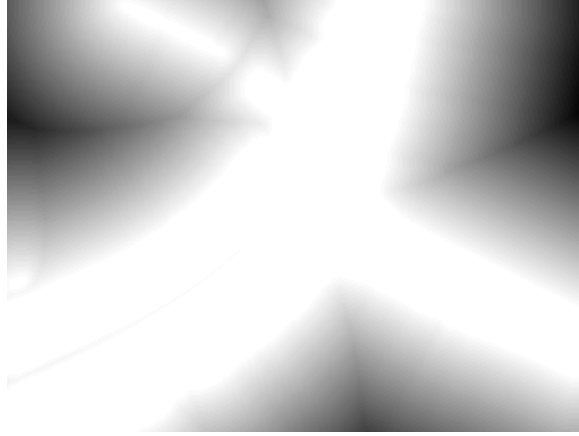
Figure 2.13: An image of N(x, y) used in the computation of E_{off-road} . This image is zero (white) on the road. For pixels that are not on the road the distance from the pixel to the closest point on the road is used as the value.
