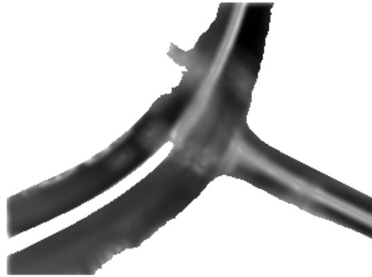
Figure 2.15: The set of seed locations for a traffic scene. The darker the pixel location, the more consistent the spatio-temporal derivatives in the region are and the better it is as a start location for a snake.
